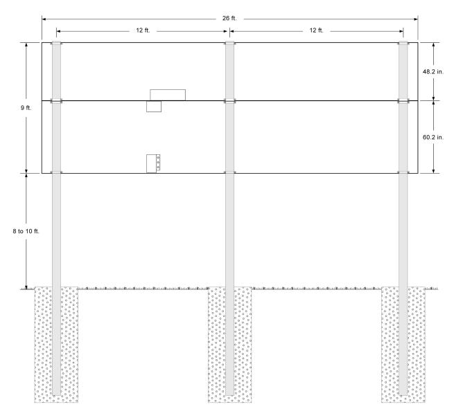
Once you have verified the positions of the posts and the size of the footings, you are ready to dig your holes, pour your concrete, and set your posts. There are several techniques for ensuring proper alignment of the posts. Typically installers will construct a temporary wooden support frame to hold each post in place while the concrete sets. Having plumb posts in the proper position is the key to a smooth mechanical installation.
